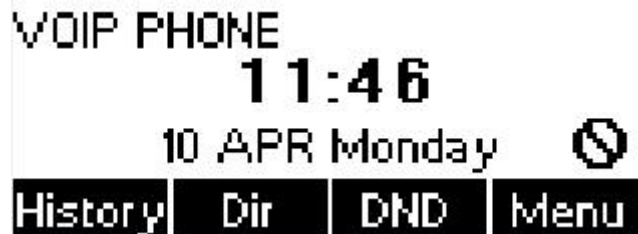
Figure 56 - DND Enabled on All Lines
